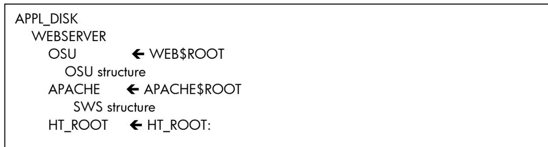
The next point was to map the structures for the web server in such a way that it would be identical for each of them: Each web server needed to see the identical structure. That meant only a single CGI procedure could handle all requests. Another requirement was that the URL used could not contain any data that was specific for one server, implying that any differences would need to be handled by the CGI procedure. Furthermore, changing the URL was out of the question.
