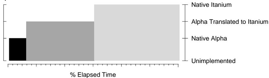
**Figure 8 – An individual application or shareable image component of an application can be transitioned from Alpha to HP Integrity systems in stages, from image translation to native execution. This allows users to be transitioned from Alpha servers to HP Integrity servers without the need to recompile code.**
