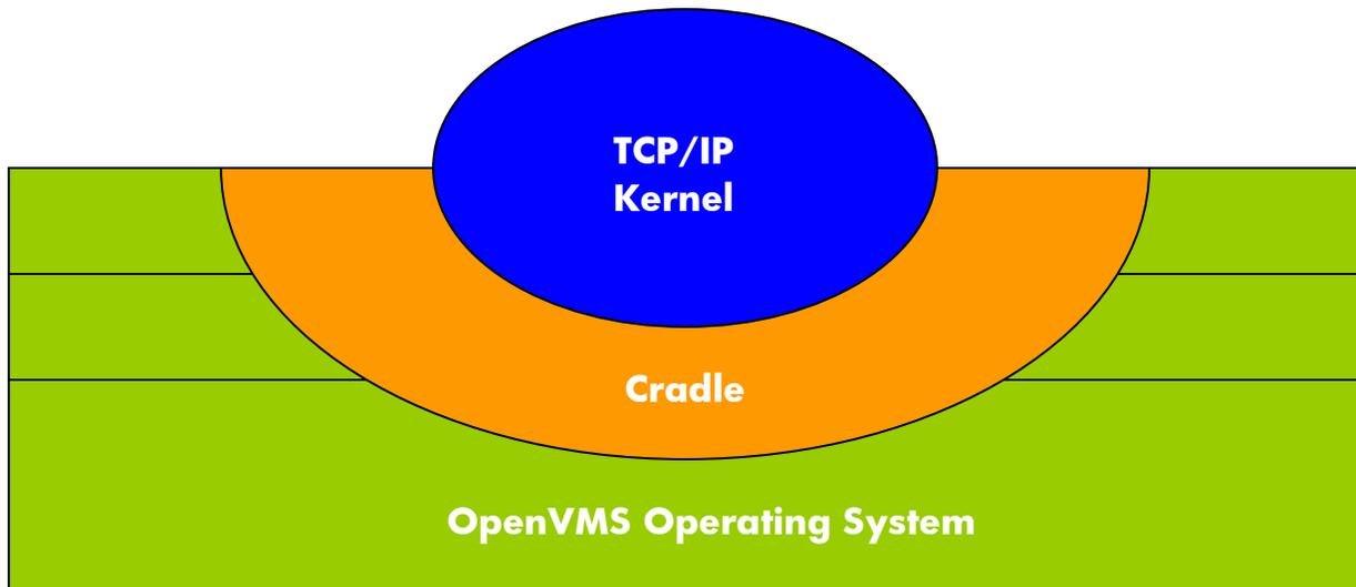
**Figure 1 The Architecture of the TCP/IP Kernel**
