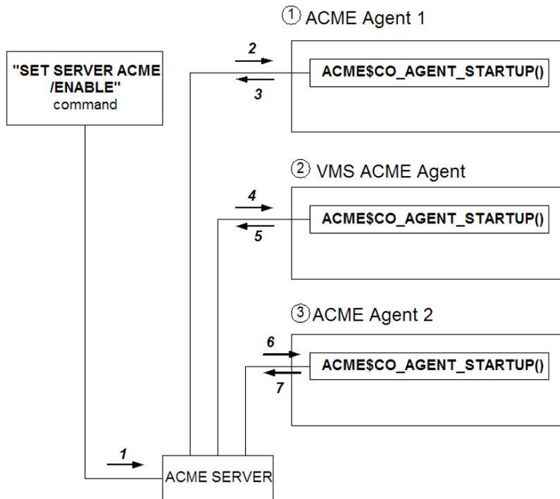
**Figure 3: ACME Control Flow for ACME\$CO\_AGENT\_STARTUP**
